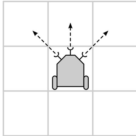
**Figure 1: Implementing sensing in Braitenberg vehicles with NetLogo.**
